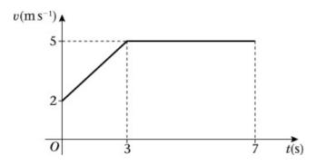
The figure shows the speed–time graph of a cyclist moving on a straight road over a 7 s period. The sections of the graph from t = 0 to t = 3, and from t = 3 to t = 7, are straight lines. The section from t = 3 to t = 7 is parallel to the t-axis.
