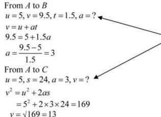
You need to find the acceleration, *a*, first by considering the motion from *A* to *B*. Then you can proceed to find the speed at *C* by considering the motion from *A* to *C*.
