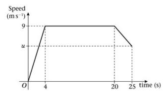
A sprinter runs a race of 200 m. Her total time for running the race is 25 s. The figure is a sketch of the speed-time graph for the motion of the sprinter. She starts from rest and accelerates uniformly to a speed of 9 m s<sup>-1</sup> in 4 s. The speed of 9 m s<sup>-1</sup> is maintained for 16 s and she then decelerates uniformly to a speed of u m s<sup>-1</sup> at the end of the race. Calculate
