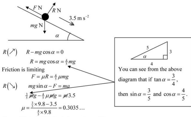
The coefficient of friction between the particle and the plane is 0.30 (2 s.f.).
