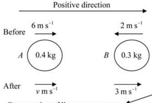
The total linear momentum before impact must equal the total linear momentum after impact.
