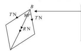
At B, the string exerts two forces, each of magnitude T. The resultant force bisects the angle ABC, which is  $80^{\circ}$ . Its magnitude can be found by resolving the two forces along the diagonal of the rhombus.
