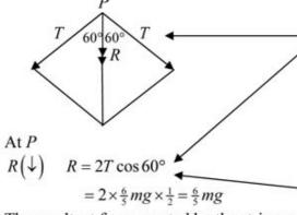
At P, the string exerts two forces, each of magnitude  $\frac{6}{5}mg$ , on the pulley both at an angle of  $60^{\circ}$  to the vertical. By symmetry, the resultant force acts vertically downwards. Its magnitude can be found by resolving the two forces vertically downwards.
