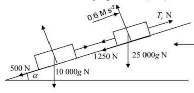
In this diagram, only the forces which are relevant when resolving up the plane have been labelled. The tractive force has been labelled  $T_r$  N.
