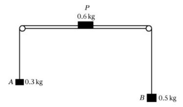
The figure shows a block P of mass 0.6 kg resting on the smooth surface of a horizontal table. Inextensible light strings connect P to blocks A and B which hang freely over light smooth pulleys placed at opposite parallel edges of the table. The masses of A and B are 0.3 kg and 0.5 kg respectively. All portions of the string are taut and perpendicular to their respective edges of the table. The system is released from rest. Calculate
