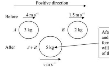
After the collision A (of mass 3 kg) and B (of mass 2 kg) combine to form a single particle. That particle will have the mass which is the sum of the two individual masses, 5 kg.
