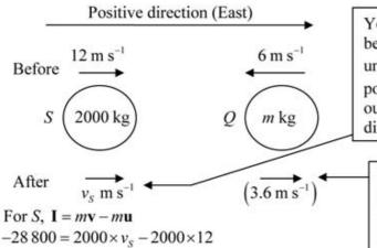
You do not know which direction S will be moving in after the impact. Mark the unknown velocity as  $v \text{ m s}^{-1}$  in the positive direction After you have worked out v, the sign of v will tell you the direction S is moving in.
