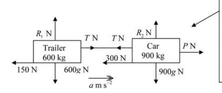
The tractive force exerted by the engine of the car has been called *P* N. This only acts on the car. It does not act directly on the trailer. The only force moving the trailer forward is the tension in the tow bar.
