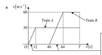
Train *B* accelerates at the same rate as Train *A*. So if Train *A* takes 12 s to reach  $30 \text{ m s}^{-1}$ , then Train *B* will take 24 s to reach  $60 \text{ m s}^{-1}$ .
