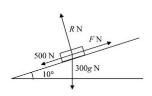
The weight has components parallel and perpendicular to the plane
