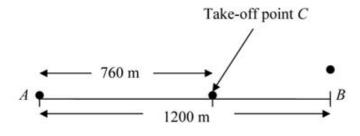
The distance AC is 760 m. The distance BC is (1200-760) m = 440 m. The aircraft takes off 760 m from its starting point A. The runway is 1.2 km, which is 1200 m, long. So the aircraft is (1200-760) m from the end C of the runway.
