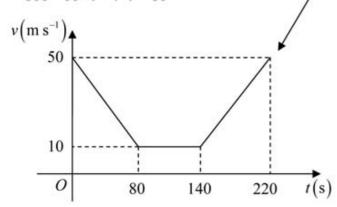
The total distance travelled is represented by two trapezia with dimensions
