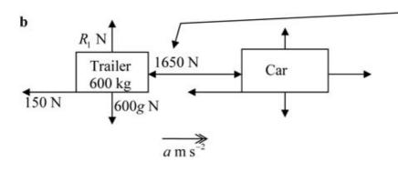
When decelerating the force in the tow bar becomes a thrust. The question gives that the greatest magnitude of the thrust is 1650 N. To solve part **b**, you need only the horizontal forces on the trailer.
