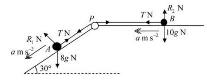
The magnitude of the acceleration of B is  $2.2 \text{ m s}^{-2}$  (2 s.f.).
