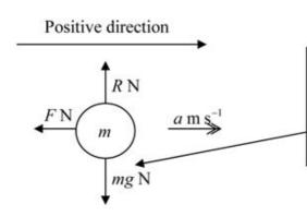
You are given no value for mass of the small stone and you will need to have an expression for the weight of the stone. Let the mass of the stone be  $m ext{ kg}$ , then the weight of the stone is  $mg ext{ N}$ .
